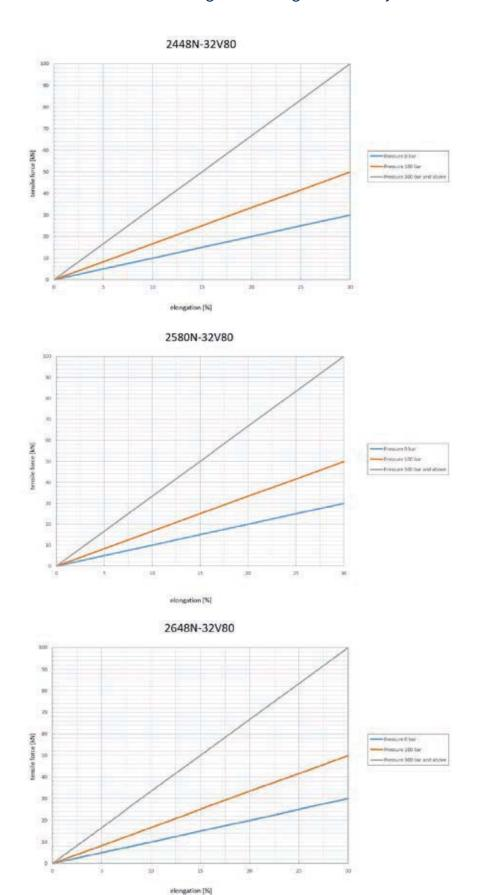
Appendix 2: Data for Tensile Loading and Weights of Polyflex Hoses
